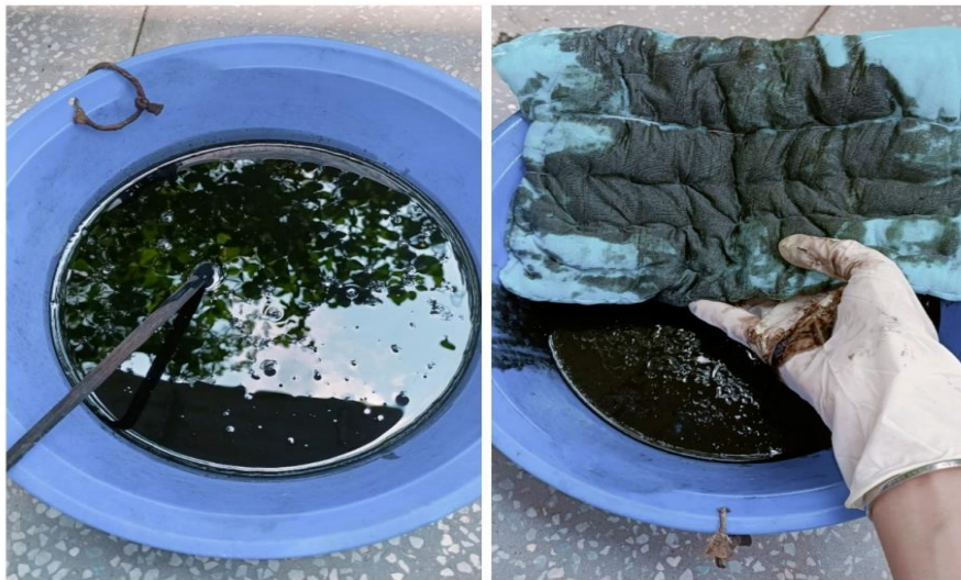
Figure: The water tank has oil scum before being treated with a mesh bag (mesh cloth) and After being treated with a mesh bag (mesh cloth)
