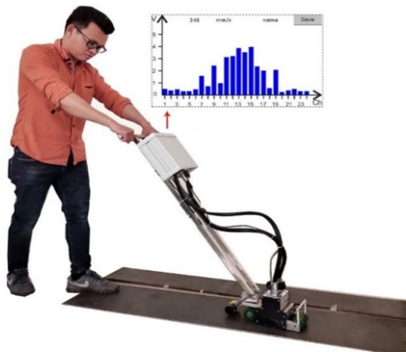
Figure 7. Experimental survey of MFL equipment on carbon steel plate
