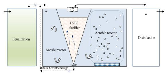
Figure 1. USBF bioreactor of Le Meridien Saigon Hotel.
