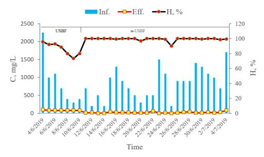
Figure 3. Suspended solids (SS) removal.
